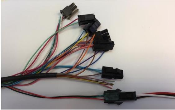
Plug the CB001 cable into the matching connector on the CB243
