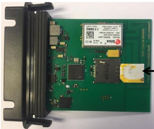
Note that the AT240 powers up when the SIM is fitted
