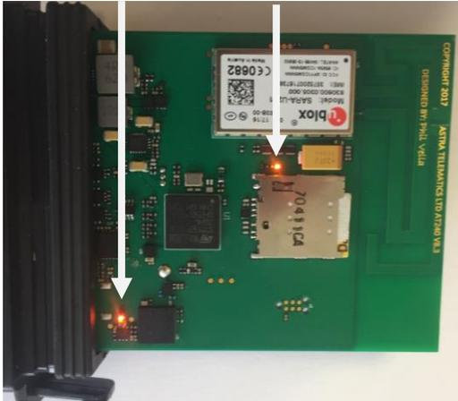
During normal operation the LEDs should appear as below:
