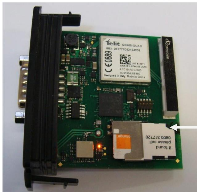
Note that the AT210 powers up when the SIM is fitted
