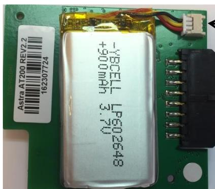
← check that battery is plugged in here
